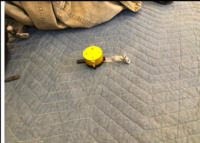
Photo 9: Field blank sample (no air pump) placed on kitchen island
