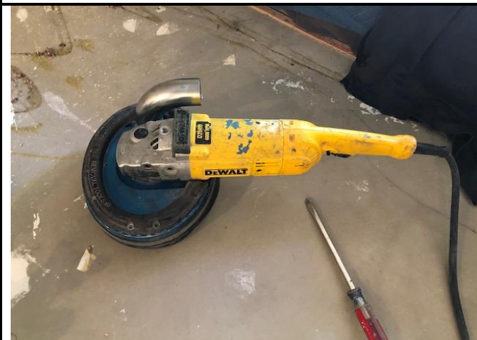
Photo 11: Example of concrete grinder with debris collection attachment
